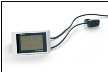
Although the control unit is designed to be mounted on the left side of the handlebar, it can also be mounted on the right. The control elements (e.g. gears) may have to be mounted on the opposite side.
