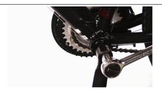
b) Remove the pedal arm with the pedal arm remover tool.
