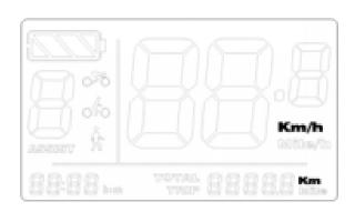
Then press (+) and (-) and no release, meanwhile press  $\mathbf{M}$  eight times, to advanced setting.
