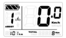
Secondly, press "+" add up speed level, press "-" cut down speed level.
