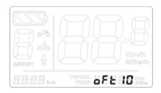
Display will sleep and cut off power after no operation on system for the setted time. Press  ${\bf M}$  to save and skip to level amount setting.
