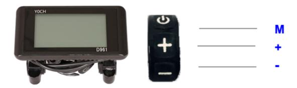
Display area includes battery capacity, riding mode, riding speed, single riding distance, total riding distance, and malfunction code of the electronic control system. Display area is as below:
